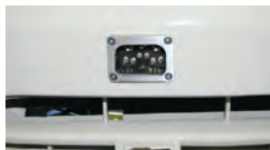
Fast Charge Port (TC022) Recharge vehicle from 30% to 80% SOC in approximately 30 minutes: For use with Off-Board Fast Charging Unit (TC033)
